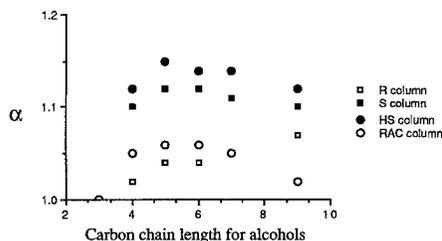
Fig. 5. Plot showing the effect of alcohol chain length on selectivity ( $\alpha$ ) for the 3,5-dinitrophenyl carbamate derivatives. □ = R column; ■ = S column; ● = HS column; ○ = RAC column.
