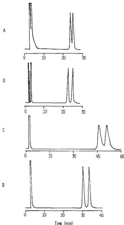
Fig. 1. Chromatograms showing the effect of %C loading on the resolution of the 3,5-dinitrobenzamide derivative of *DL*-phenylalanine on: (A) the R column; (B) the low-load S column; (C) the high-load S column and (D) the racemic column. Mobile phase conditions are as specified in Table II.
