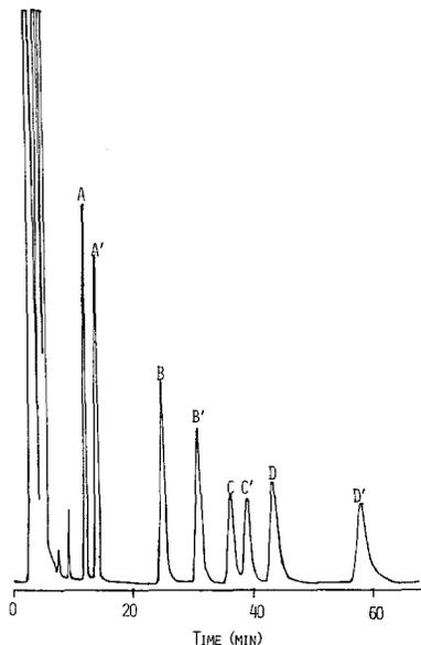
Fig. 2. Chromatogram on the low-load S column showing the enantiomeric separation of the 3,5-dinitrophenyl derivatives of: (A) 4-methyl-2-pentanol; (B) 1,2,3,4-tetrahydro-1-naphthol; (C) *sec*-butyl amine and (D) 2-phenylpropionic acid. Mobile phase: isopropanol-hexane (10:90) at 1 ml/min; UV detection at 254 nm.
